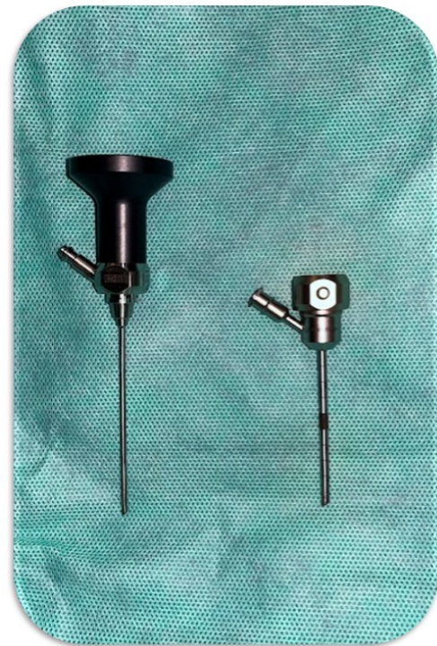
Figure 8. The 1.9-mm Nexus Scope is 115 mm long with a 63.1 mm working length, a 65-degree field of view, and a 30-degree direction of view. The accompanying 1.9 mm Warburton Collar-lock Scope Cannula is 50 mm long, marked for a 25 mm working length for scope or portal use.
